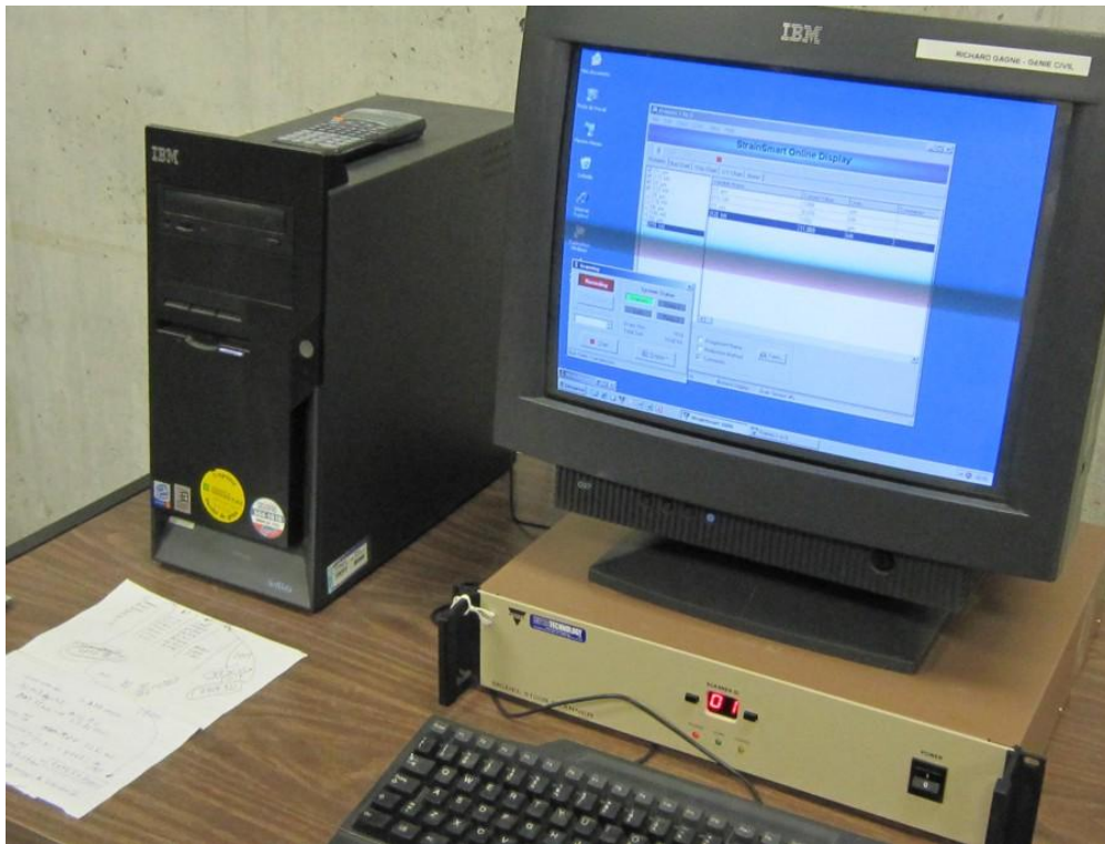
Figure 3. VISHAY System 5100B data acquisition system
