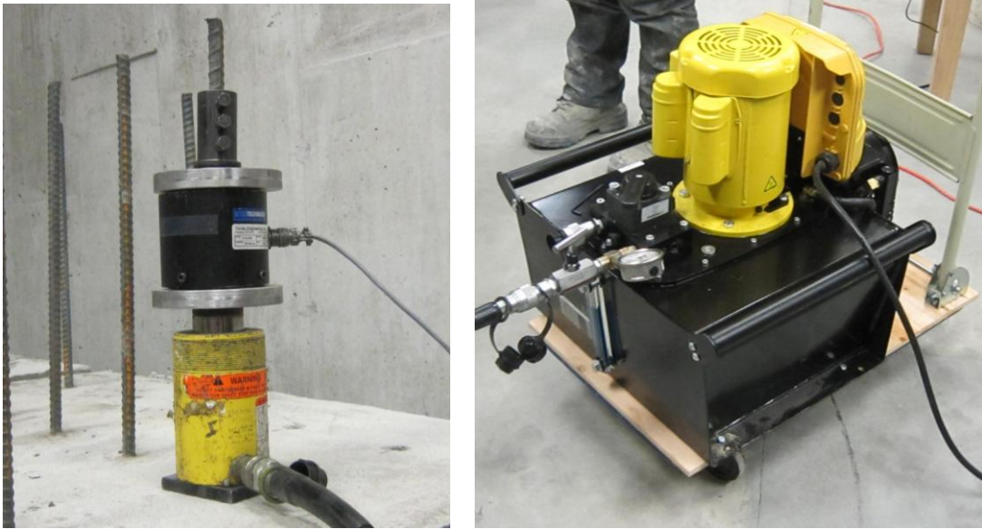
Figure 5. Static load testing setup
